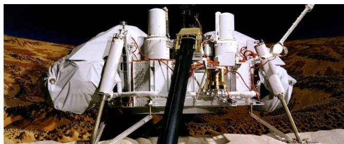
Figure 3: Viking lander, the first spacecraft to reach the surface of Mars where it searched for biosignatures. Image credits: NASA Astrobiology.
